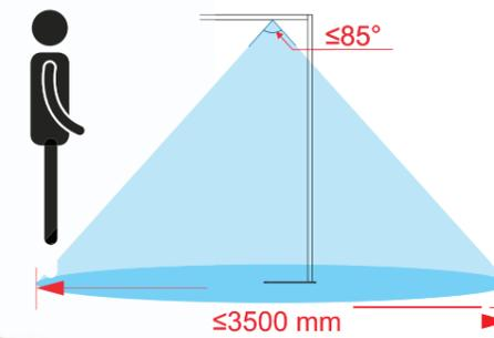
Here to tell you how to play Motion Sensor & Daylight Sensor
