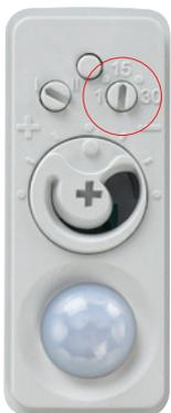
The ActiLume I-10V Sensor has the option to set the delay time between last moment of presence detection and starting the “Exit” sequence. During the Exit sequence of approximately 15 seconds, the lights will gradually dim down to the minimum level which is a dimming voltage of 2.5V. The sensor cannot dim below 2.5V due to the fact that there is a micro-processor inside the sensor that will stop functioning if the dim voltage drops below 2.5V.
