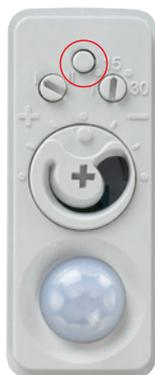
On the sensor, there is a pushbutton to activate/deactivate the 100 hours burn in sequence.
