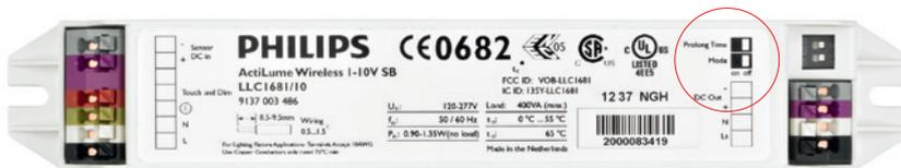
Switch 1 is called Mode and it will give the possibility to change the daylight-override between 150% (Mode 1 – Switch 1 is set to off) or 250% (Mode 2 – Switch 1 is set to on). If the luminaire(s) are switched off due to excessive daylight, then, as soon as the light level goes below 100%, the Wireless SwitchBox will switch on the luminaire(s) again.
