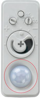
The movement sensor is a PIR (Passive Infra-Red) sensor that detects occupancy with an X-Y cross-area under an angle of  $X = 81^\circ$  and  $Y = 95^\circ$ . When installed in a typical office ceiling at 2.5 meter height, it is sensitive to small movements within a 4 by 6 meter area. It will cover small movements down to a few centimeters at the task area of a desk and is sensitive to large movements within a range of 6 by 7.5 meters. See also figure below.
